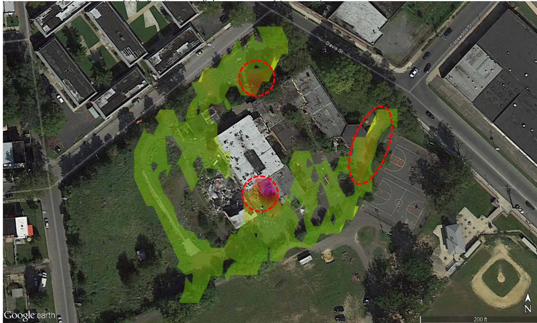
Conductivity[500InPhase[10000] 2011 Google Imagery Areas of near-zero positive conductivity (light green), areas of high positive conductivity (warm colors)
