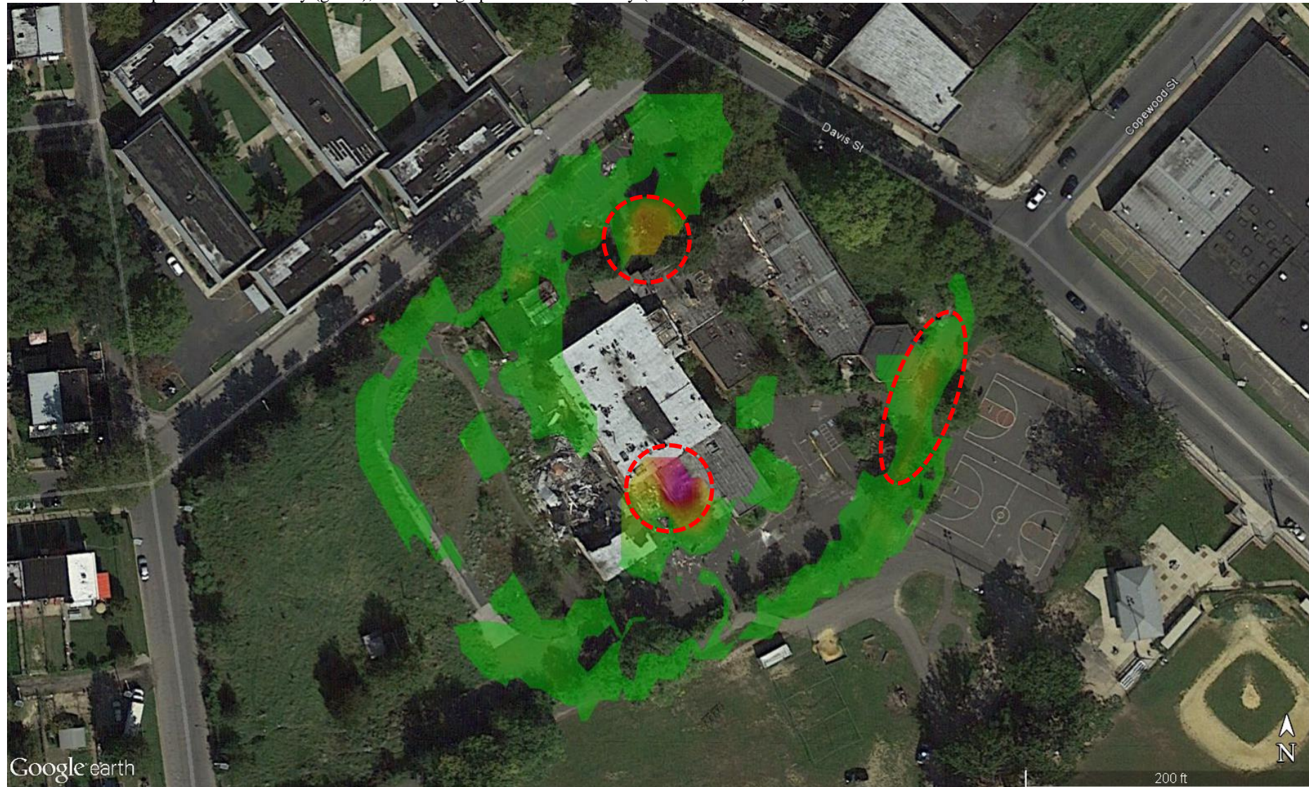
Conductivity[100InPhase[15000] 2011 Google Imagery Areas of near-zero positive conductivity (green), areas of high positive conductivity (warm colors)
